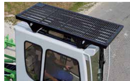
Bulletproof windshield and skylight are now standard on all new SENNEBOGEN material handlers.
