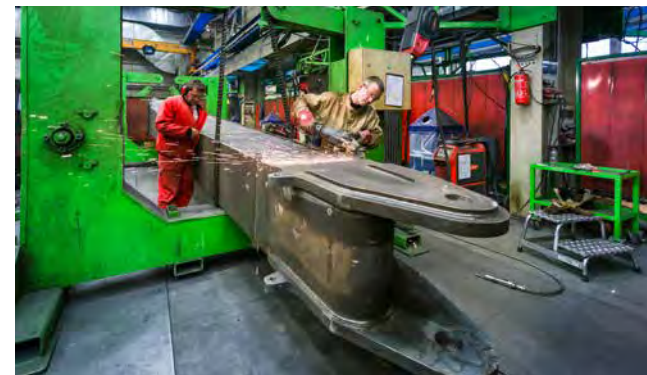
The upper carriage is built around a large, continuous one-piece center frame for added structural strength and improved air flow.
