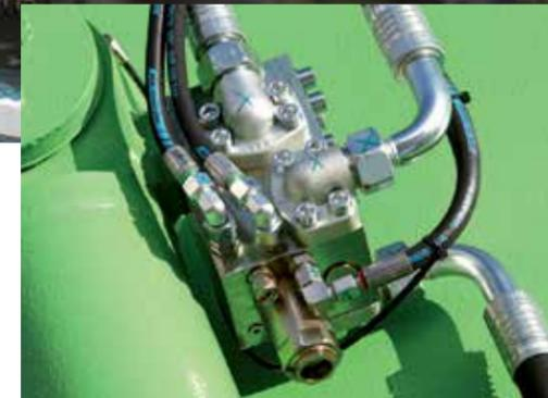
With hydraulic controls instead of electronics, the 718 requires no special software or "black box" components to troubleshoot your machine.
