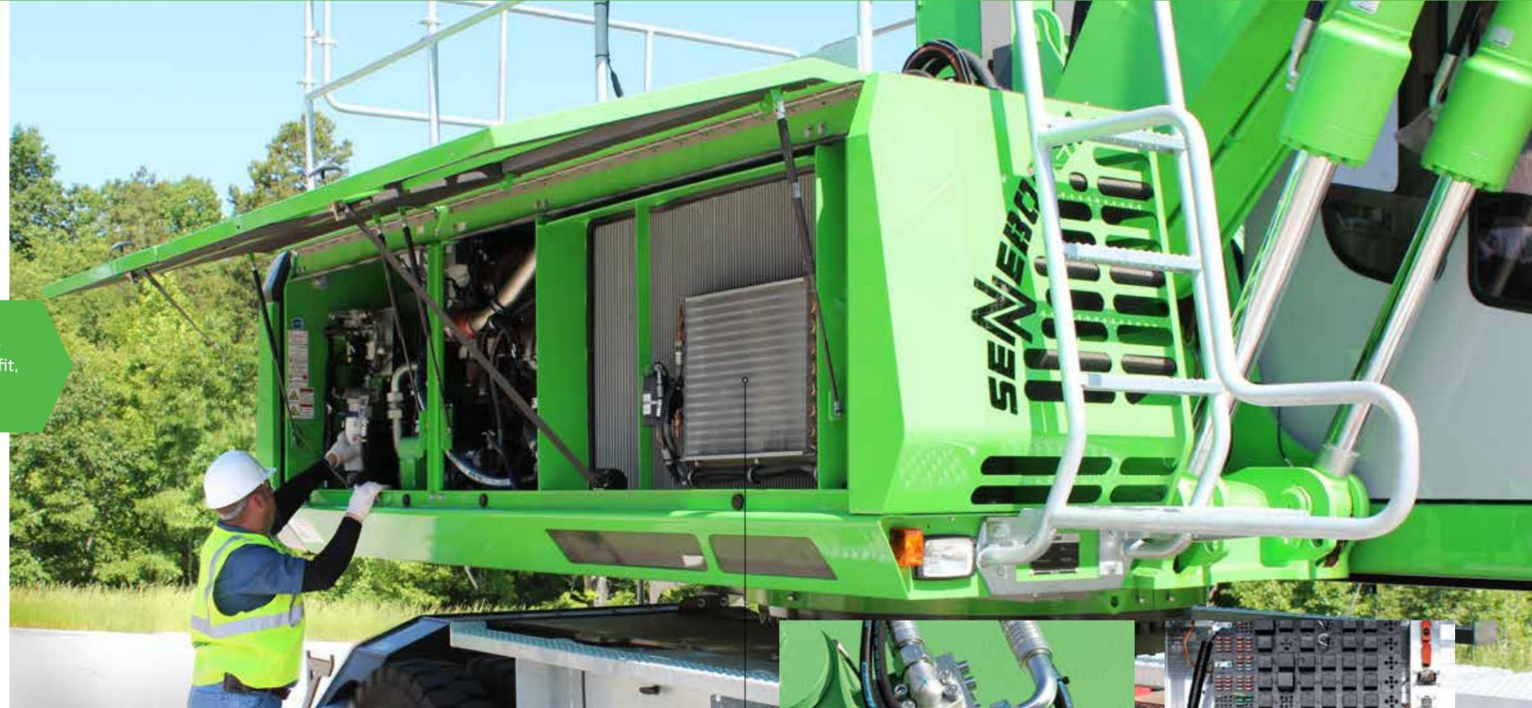
Natural airflow through the engine compartment, uninterrupted from front to back, plus a large reversing cooling fan, lets your 718 start reliably and keep on running through any extremes of heat, cold or dusty conditions.
