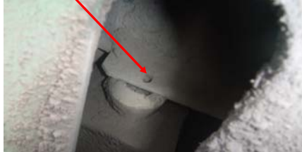
Bolt is missing on the hydraulic filter
