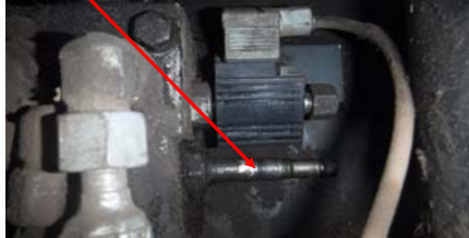
Park brake coil is missing.
