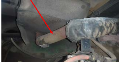
Exhaust insulation is missing.
