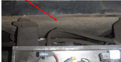
Exhaust insulation is missing.
